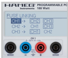
Individual Linking of single Channels using FuseLink
