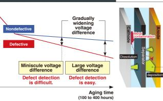
Since the amount of change in OCV caused by self-discharge is extremely small, it is necessary to age batteries at least 100 to 400 hours before testing can accurately distinguish between non-defective and defective products. Additionally, it is necessary to measure OCV multiple times during the aging process. Using an instrument with good accuracy makes it possible to remove defects from the testing line earlier in the process, significantly reducing management and testing costs.
