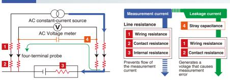
High line resistance can cause current errors and measurement errors, preventing accurate testing
