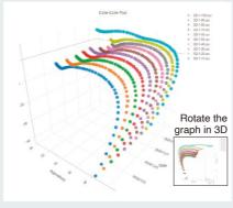
Bode plots, using the time or date as a third axis. Rotate 3D graphs in any direction as desired and save images.
