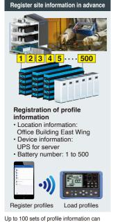
be registered on the BT3554-50. Up to 500 data sets can be saved for each profile. (The BT3554-50 can save up to 6,000 data
