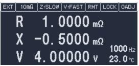
Measure 4-V Li-ion battery cells at an accuracy of ±190 µV
