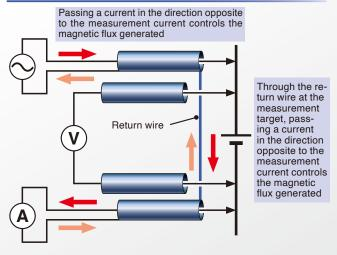
2. The magnetic flux generated by the eddy current generates induced voltage in the voltage terminal
