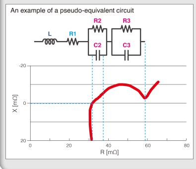
The impedance characteristics of a Cole-Cole plot are generally expressed as a pseudo equivalent circuit.
