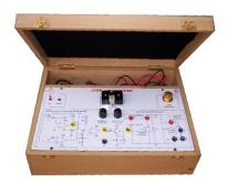
Step up Chopper designed to study stepping up of voltage by change in duty cycle of the pulse at the gate of mosfet.
