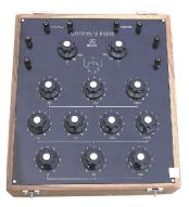
• To calculate the value of unknown Inductance in terms of Capacity and Resistance.
