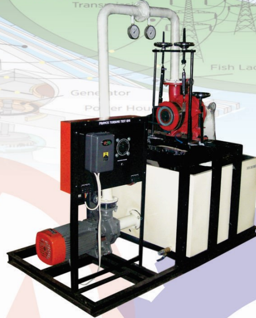
GN 7278 - Francis Turbine Test Rig
