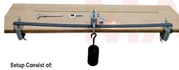
· Two parallel knife edges on which the beam is placed
