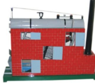
BABCOCK AND WILCOX BOILER
